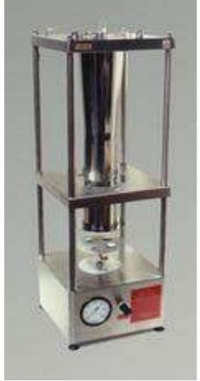
pneumatic on/off switch mounted outside Potter Precision Laboratory Spray Tower (Manual load) (make-Burkard Scientific, England)
