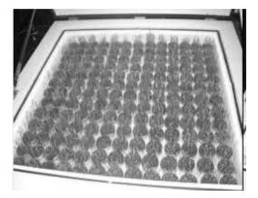
Thermogradient plates are set up in different ranges of temperature and this determines the exact temperature required for the germination of seeds. The gradient variation in temperature in sections is  $0.5^{\circ}$ C or 1°C.
