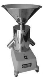
It is used for dividing and mixing of seed/grain which do accurate division and reduction to working size of samples exactly representative of the original sample.
