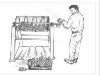
Net drum rotator used for separation of seeds of conifers
