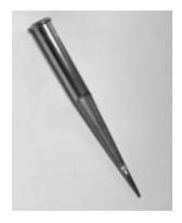
It is used for sampling seed from bag but not in bulk. It is inserted pointing upwards at an angle of about 30° to the horizontal, with the hole facing downwards until it reaches the centre of the bag, then revolved through 180°, bringing the hole face upwards, and is withdrawn with decreasing speed so that the quantity of seed obtained from successive locations increases progressively from centre to side of the bag.
