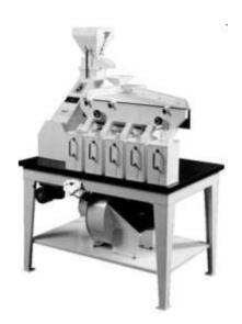
and particles of inert matter at the top and the heaviest at the bottom. An oscillating movement of the table causes the seeds to move at different rates across the deck. The lightest seeds float down under gravity and are discharged at the lower end, while the heaviest ones are kicked up the slope by contact with the oscillating deck and are discharged at the upper end.
