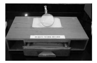
It is the instrument used for separating the inert matters from the seed samples. Inert matters can be anything other than the seeds like parts of leaves, stems, chaff, twigs, soil material, discolor and 10ther foreign materials.
