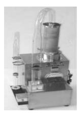
The seed blower serves for quick and easy separation of light and heavy fractions of a great variety of seeds. The blower is equipped with a synchronous motor to ensure uniform RPM and air flow is regulated with a calibrated vernier gate.
