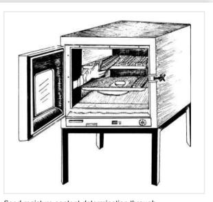
Seed moisture content determination through oven dry method
