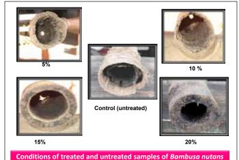
Conditions of treated and untreated samples of *Bambusa nutans* removed after 12 months
