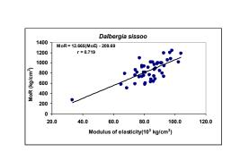
Fig.- 3. Modulus of rupture as a function of modulus of elasticity.
