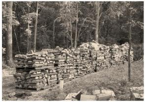
The process of inducing evaporation of the moisture contained in wood; a type of hydrothermal treatment of wood is known as wood seasoning.
