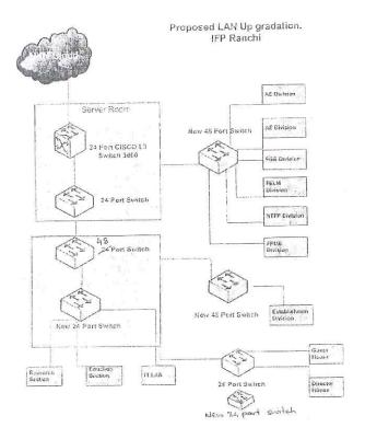
New 24 port Switch will be installed and connected with Research Section. Education Section and IT LAB by replacing all the HUBS
