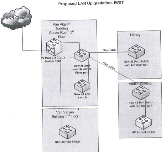
New one 46 port switch having 2 fiber port and one new 24 port switch added to Va Vigyan building 3<sup>rd</sup> floor by replacing old three 24 port switches
