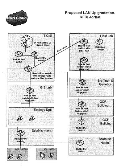
In IT- cell 4 24 port Dlink Switches will be replaced with 2 Nos, 48 Port switches. One 24 port dlink switch replaced with 1Nos, 24 port switch with all Giga port.
