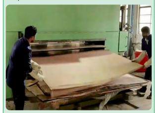
Unloading plywood made using Phenol lignin formaldehyde resin
