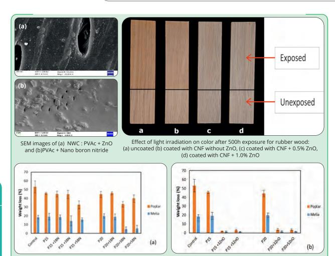
Decay resistance of wood and NWC against brown rot fungus (a) PVAc with boron nitride; (b) PVAc with ZnO
