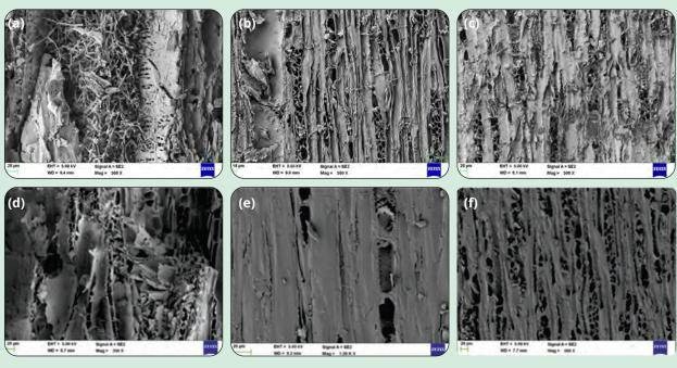
SEM images of untreated and nanoemulsion treated specimens after exposure to white rot fungi (a-c): (a) untreated wood, (b) NE with nanoZnO treated wood, and (c) NE with nanoCuO treated wood; specimens exposed to brown rot fungi (d-e): (d) untreated wood, (e) NE with nanoZnO treated wood, and (f) NE with nanoCuO treated wood.
